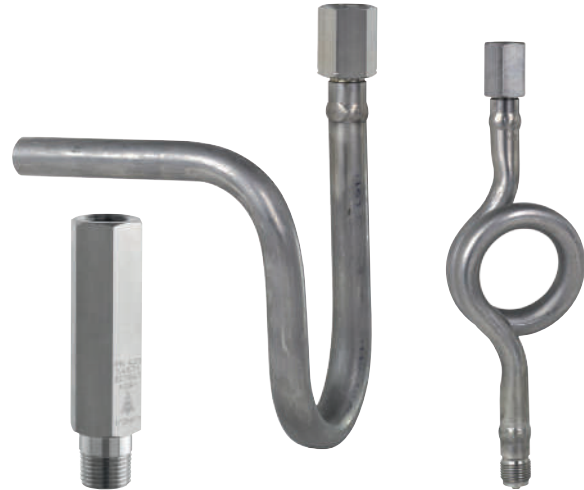
Syphons, model 910.15, stainless steel Fig. left: Compact form Fig. centre: U-form, DIN 16282 form B Fig. right: Trumpet form, DIN 16282 form D
