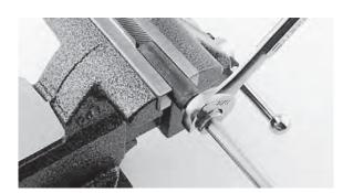
Place Pre-Set Tool in a vice and tighten nut specified number of turns.
